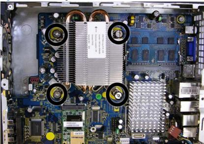
Figure 7-32 Removing the heat sink
